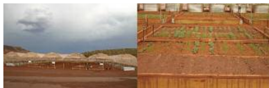
Left - the recently completed RSB controlled environment facility (CEF) situated in proximity to active restoration sites. This shelter will test different restoration soil types (using up to 64 plots) and watering regimes (up to 4) that will reflect current soils available for restoration purposes as well as likely rainfall patterns seeds and seedlings may naturally experience - from extreme drought right through to above average rainfall conditions. Right - in situ emergence of Pilbara species after several weeks incubation in the CEF. (Todd Erickson)
